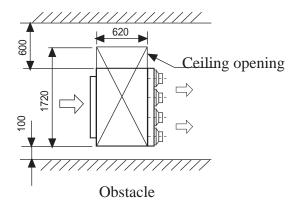
**Space installation needed (unit: mm)**
